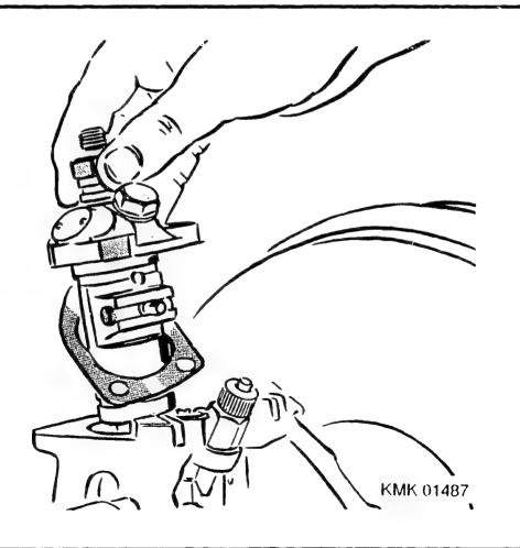
Check prestroke setting again and repeat adjustment if necessary.
